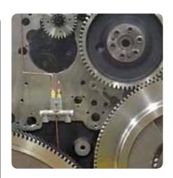
Pressure switch or transducer
