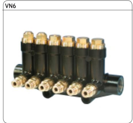
The distributors meter and distribute the lubricant from the pump to the individual lubrication points. They do so independent of each other.
