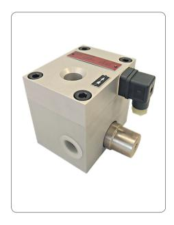
Flow limiters are used in circulating-oil lubrication systems. The task of a flow limiter is to divide up the volumetric flow of the main line into parallel individual volumetric flow quantities and to "limit" these according to requirements, or to keep them constant.
