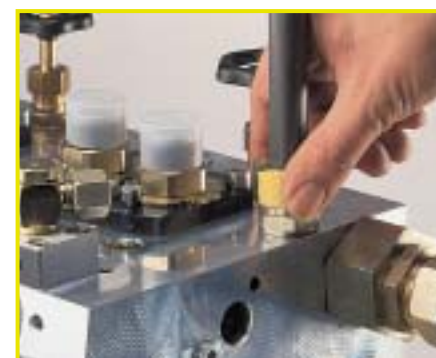
To ensure lubrication even in arctic temperatures, the lubrication pump can be connected to the main oil system of the diesel engine.
