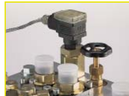
The contamination of the oil supply filter is also monitored with the level indicator switch.
