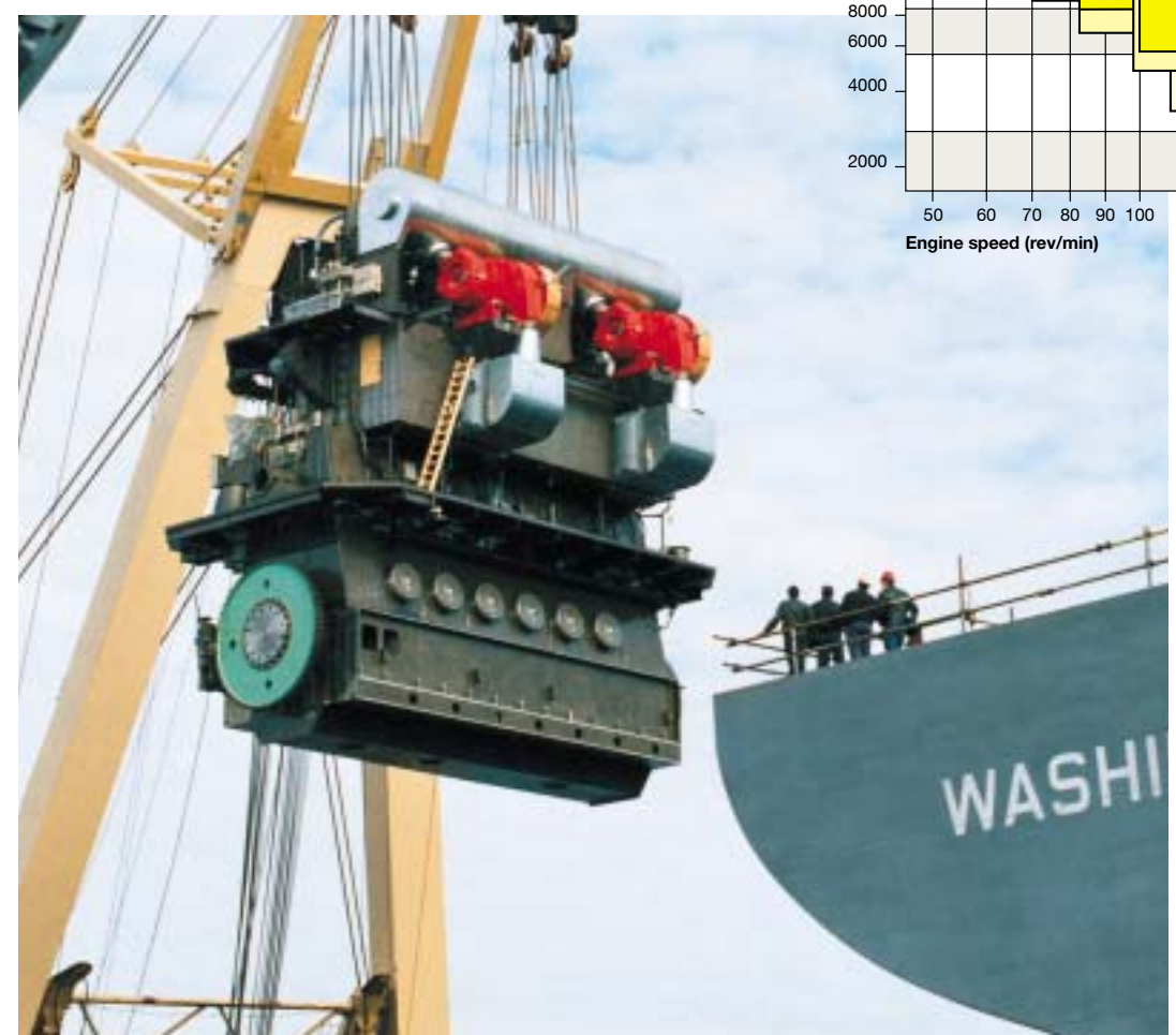
Photo: DMR-Sulzer 7RTA72U
